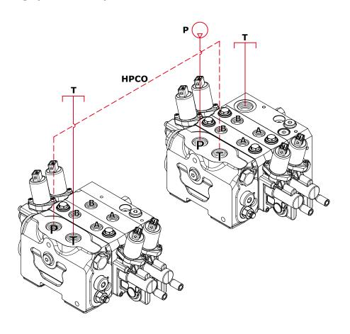
The Carry Over function is yet another unique option offered by the EX family. In fixed pump circuits, two control valves connected in succession can be used to ensure flow through both valves' inlet compensators. This special design is obtained by using a special inlet cover on the first valve. This circuit is ideally sui-
